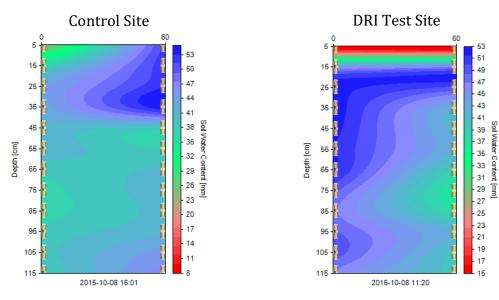
Using onsite flow meters, the DRI site demonstrated a savings of 4.54 gallons of applied water to reach a similar saturation point as in the drip control site per vine. The applied water at the DRI site was 2.84 gallons per vine, compared to 7.38 gallons per vine in the drip control site.
